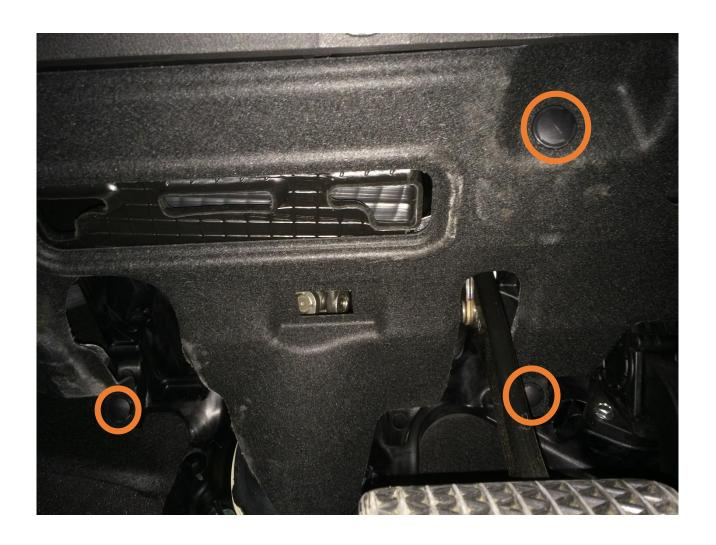
**4- Some** VF commodores have a **foot well globe** which will also need to be detached. The locations of the pop clips are **circled** below. The **foot well globe** is removable by hand when the panel is off.
