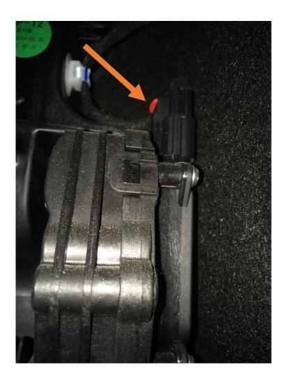
**6-** Once the pin has been pulled back, push down on the black tab **circled** below as you remove the plug.
