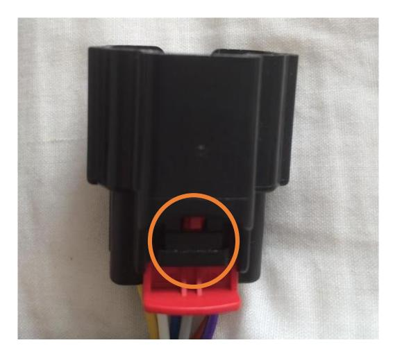
7- Using the supplied harness, plug the male to female end for both the accelerator side and the loom side. THE IMAGE BELOW IS FOR ILLUSTRATIVE PURPOSES ONLY, you do not need to remove the accelerator pedal to install the controller, this is a VE pedal for reference.
